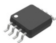
MCP4812T-E/MS Microchip Technology IC DAC 10BIT V-OUT 8MSOP
