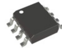
MCP4821T-E/SN Microchip Technology IC DAC 12BIT V-OUT 8SOIC
