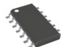
MCP4902-E/SL Microchip Technology IC DAC 8BIT V-OUT 14SOIC
