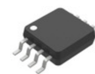
MCP4812-E/MS Microchip Technology IC DAC 10BIT V-OUT 8MSOP
