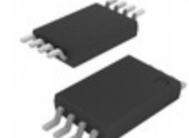
93LC56BT-I/ST Microchip Technology IC EEPROM 2KBIT MICROWIRE 8TSSOP
