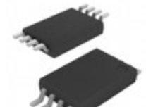
93LC56BT/ST Microchip Technology IC EEPROM 2KBIT MICROWIRE 8TSSOP
