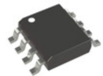
93LC56BT-I/SN Microchip Technology IC EEPROM 2KBIT MICROWIRE 8SOIC
