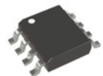
93LC56BXT-I/SN Microchip Technology IC EEPROM 2KBIT MICROWIRE 8SOIC
