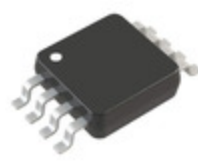
ADR443ARMZ Analog Devices Inc. IC VREF SERIES 0.13% 8MSOP
