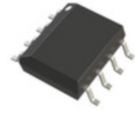
ADR440BRZ Analog Devices Inc. IC VREF SERIES 0.05% 8SOIC
