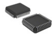
EPM3032ALC44-7N Intel IC CPLD 32MC 7.5NS 44PLCC
