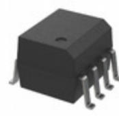
FOD0720R2 Fairchild Semiconductor HIGH CMR, 25MBIT/SEC LOGIC GATE
