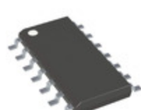
MCP6494T-E/SL Microchip Technology IC OPAMP GP 4 CIRCUIT 14SOIC
