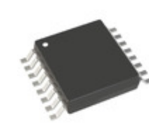
AD7798BRUZ-REEL Analog Devices Inc. IC ADC 16BIT SIGMA-DELTA 16TSSOP
