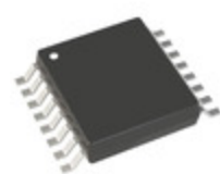
AD7798BRUZ Analog Devices Inc. IC ADC 16BIT SIGMA-DELTA 16TSSOP
