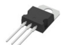
STP5N120 STMicroelectronics MOSFET N-CH 1200V 4.7A TO220-3
