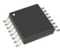
AD5142ABRUZ100-RL7 Analog Devices Inc. 256TAP, DUAL DIGIPOT, NVM, I2C
