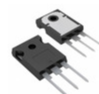
STW25NM60N STMicroelectronics MOSFET N-CH 600V 21A TO247-3
