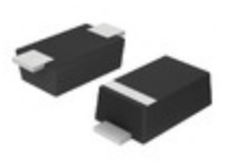
NRVBAF260T3G onsemi DIODE SCHOTTKY 60V 2A SMA-FL
