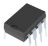
ADP667AN Analog Devices Inc. IC REG LDO 5V OR ADJ LIN 8-DIP
