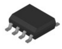
MPXV5004GVP Freescale Semiconductor SENSOR 0.57PSIG 0.13" 4.9V 8SOP
