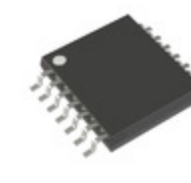
PIC16LF1824-I/ST Microchip Technology IC MCU 8BIT 7KB FLASH 14TSSOP
