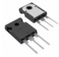
STGW35HF60WD STMicroelectronics IGBT 600V 60A 200W TO-247
