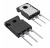
STGW30NC120HD STMicroelectronics IGBT 1200V 60A 220W TO247
