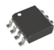
25A512-I/SN Microchip Technology IC EEPROM 512KBIT SPI 8SOIC
