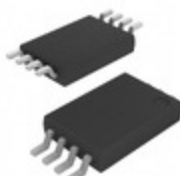
25AA010AT-I/ST Microchip Technology IC EEPROM 1KBIT SPI 10MHZ 8TSSOP
