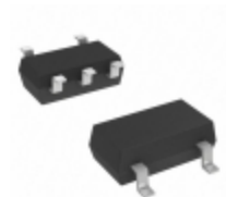
TSV611ICT STMicroelectronics IC OPAMP GP 1 CIRCUIT SC70-5
