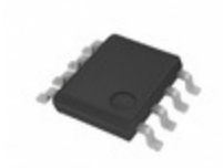
TSV612AIST STMicroelectronics IC CMOS 2 CIRCUIT 8MINISO
